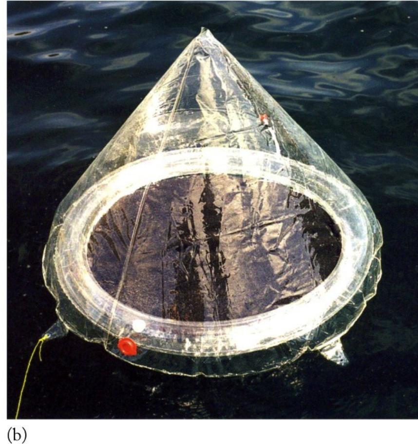
Fig. 1.8 Collection of pure water from seawater using a solar still.
