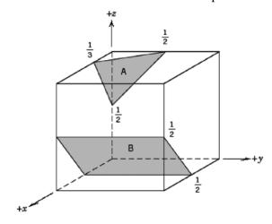
3.54 Determine the Miller indices for the plane shown in the following unit cell:
