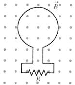
3. A uniform magnetic field  $\overline{B}$  is perpendicular to the plane of a circular wire loop of radius r. The magnitude of the field varies with time according to  $B = B_0 e^{-t/\tau}$ , where  $B_0$  and  $\tau$  are constants. Find an expression for the emf in the loop as a function of time.
