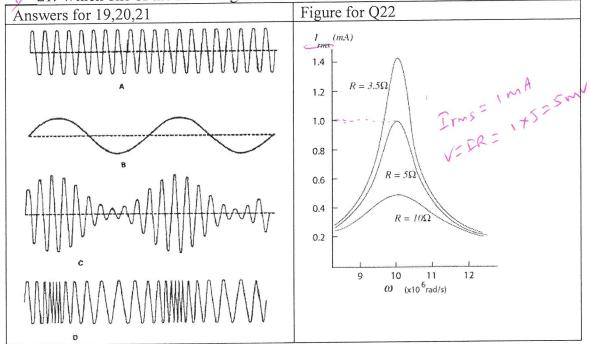
22. The resonance curves for an RLC circuit are shown for various resistances above. Using the plot, determine the V<sub>rms</sub> for the 5 ohm resistor at the resonance? f. 5.0 mV b. 0.45 mV c. 0.8 mV d. 1.0 mV e. 1.4 mV a. 0.4 mV
