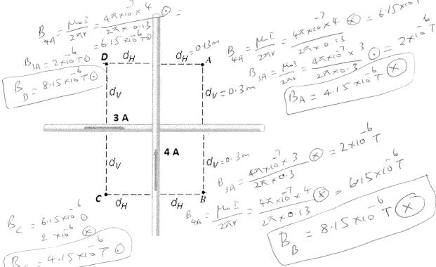
B. The magnetic field (B) due to a long straight wire, carrying a current (I), at a distance
