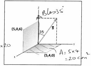
9. A loop of wire has the shape shown in the drawing. The top part of the wire is bent into a rectangle of length 0.30 m and width 0.20 m. A constant magnetic field of magnitude 0.80 T is directed into the paper. What is the change in magnetic flux when the rectangular side is rotated through ¼ of a revolution, starting from the position shown?
