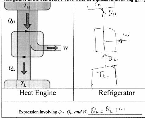
$$Q = mc\Delta T \qquad Q = mL \qquad (COP)_{Refri.} = \frac{\varrho_c}{w}$$
