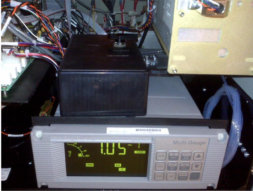
**Figure 7:** Vacuum gauge and 3-position CID box
