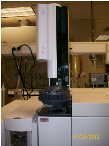
Figure 5: GC-MS, Autosampler with vial in place ready for analysis
