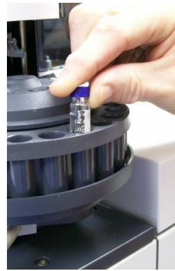
Figure 4: Placement of Vial into Autosampler
