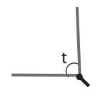
3. Use the protractor to measure the angle between the legs of the compass (Angle t).
