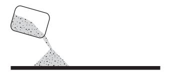
1. Slowly pour the sand onto the tray, keeping the pour spout steady in one place.
