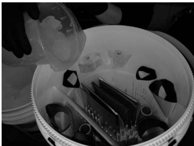
FIG. 3—Aqueous gel being placed around mock evidence arranged in a 5-gal bucket. [Color figure can be viewed at [wileyonlinelibrary.com](http://wileyonlinelibrary.com)]
