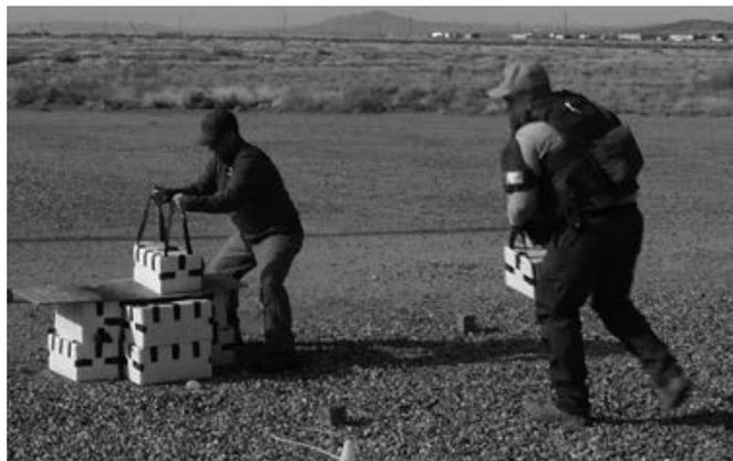
FIG. 1—Filled gel blocks may be placed around an IED to capture small shrapnel. [Color figure can be viewed at [wileyonlinelibrary.com](http://wileyonlinelibrary.com)]
