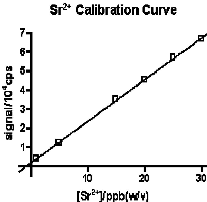
The standard calibration curve is fit with a straight line with a slope of  $0.2182 \pm 0.002239$  (s.d.) and a y-intercept of  $0.1840 \pm 0.04264$  (s.d.), with  $r^2 = 0.9996$ . The detection limit
